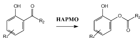
Scheme 3. Biocatalytic production of protected catechols using HAPMO.
